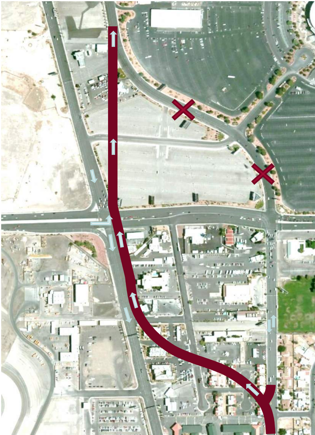
Figure 5 – Swenson Street Realignment Alternative C
