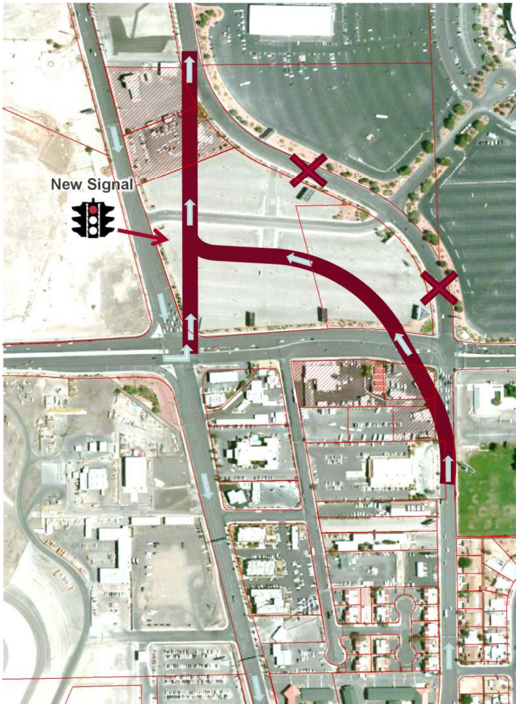
Figure 2 – Swenson Street Realignment Alternative A (Parcels Affected)
