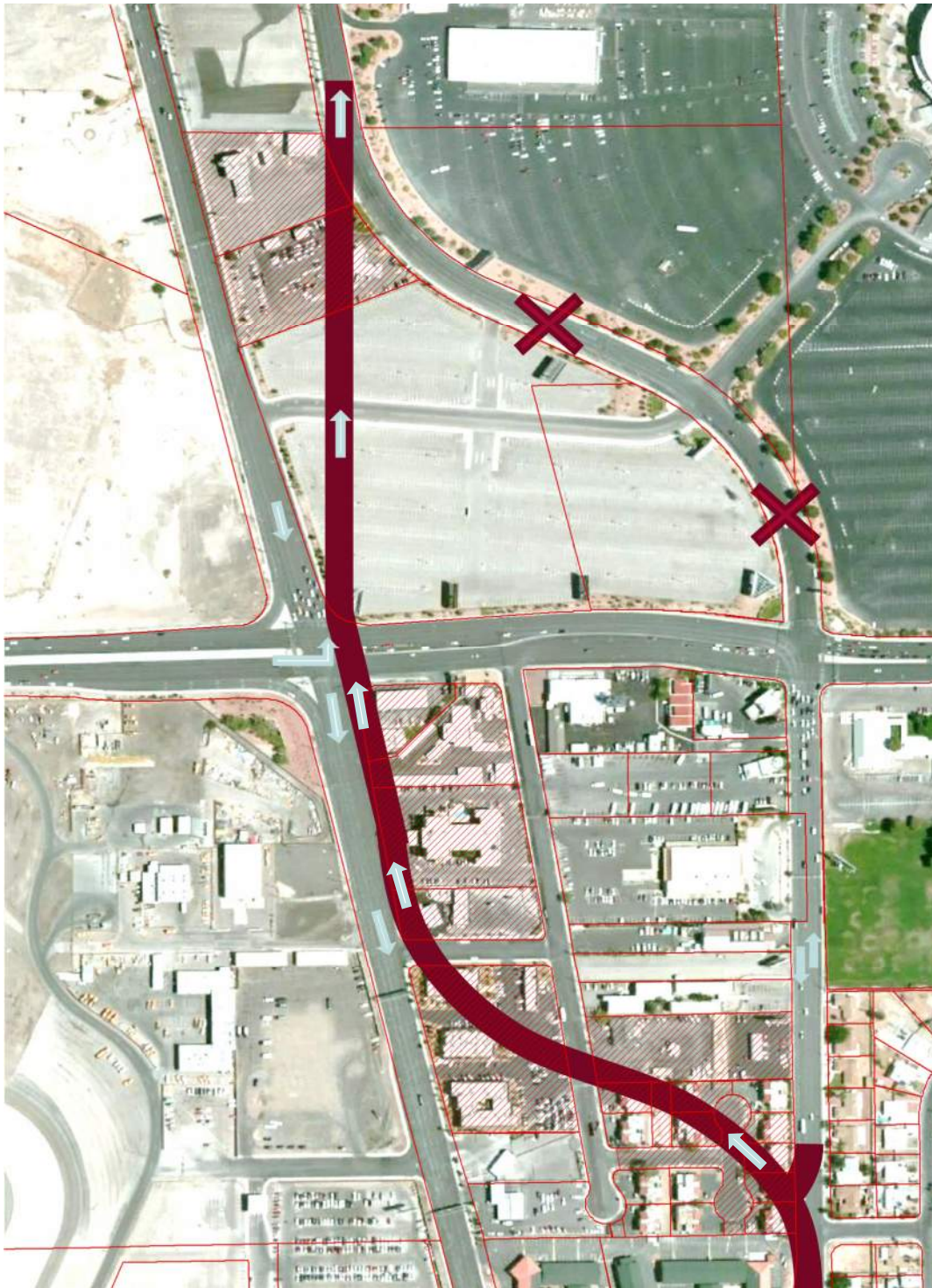
Figure 6 – Swenson Street Realignment Alternative C (Parcels Affected)
