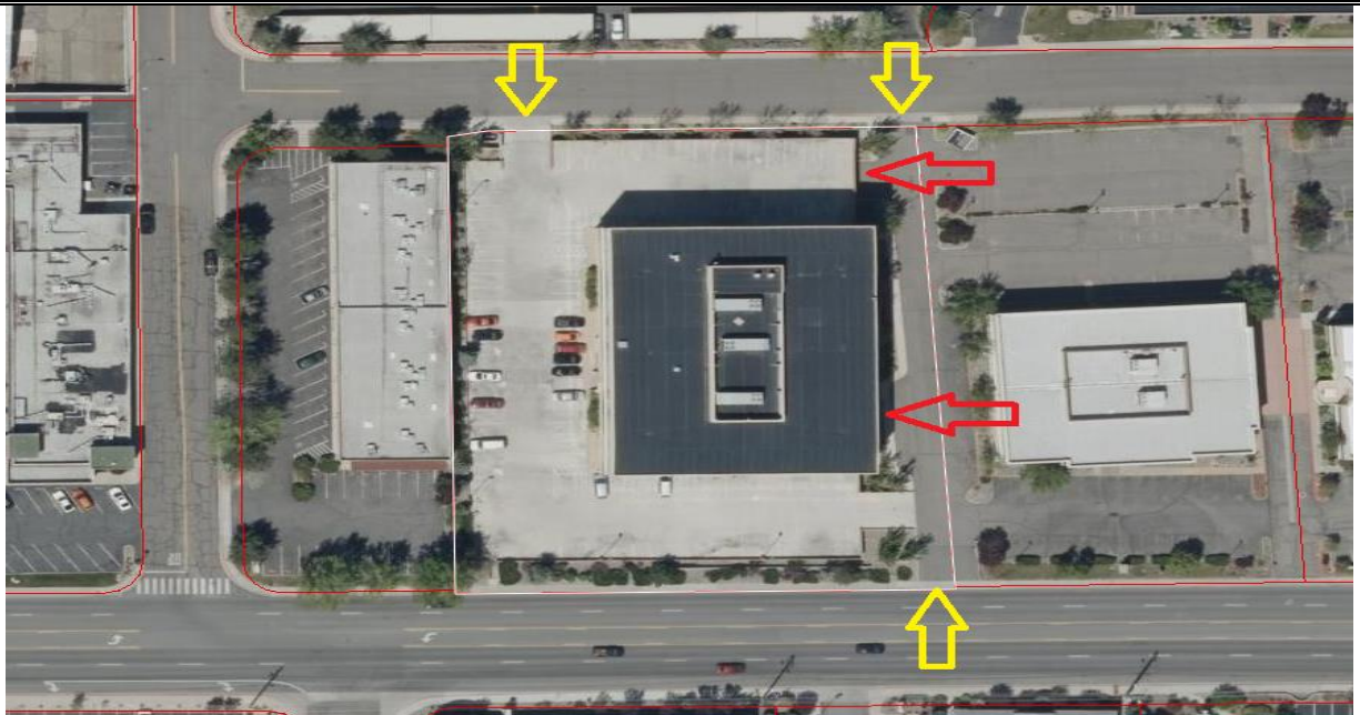
SITE VEHICULAR ACCESS POINTS DEPICTED BY YELLOW ARROWS; SUBTERRANEAN GARAGE ACCESS DEPICTED BY RED ARROWS
